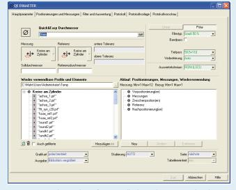
An assistant in the Mahr software called Quick&Easy guides the operator through the reference measurement and diameter determination. After the evaluation, it immediately creates the appealing and informative result record in which the roundness deviation is visually provided in addition to the diameter results.
